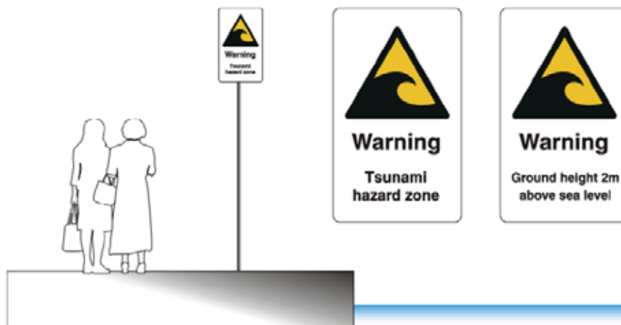
Example of ISO 20712 Tsunami Hazard Sign Placement
